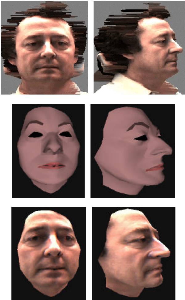
Figure 4: (Top) Frontal and side views of the texture calibration target “Claude” [13]; (center) model “Oscar” reshaped with the feature points of “Claude”; (bottom) model “Oscar” reshaped with feature points and with the texture of “Claude”.
